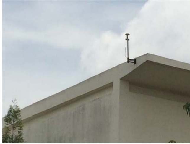
Figure 2 GPS antenna located on top of the building to avoid the multipath.
