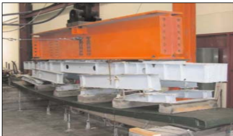
Figure 11: Proof test of Short Span FRC Bridge using whiffle tree (Robinson et al. , 2008).
