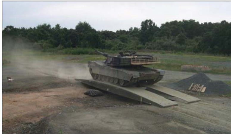
Figure 10: Field testing of CAB by MLC 100 vehicle (Robinson, 2008).
