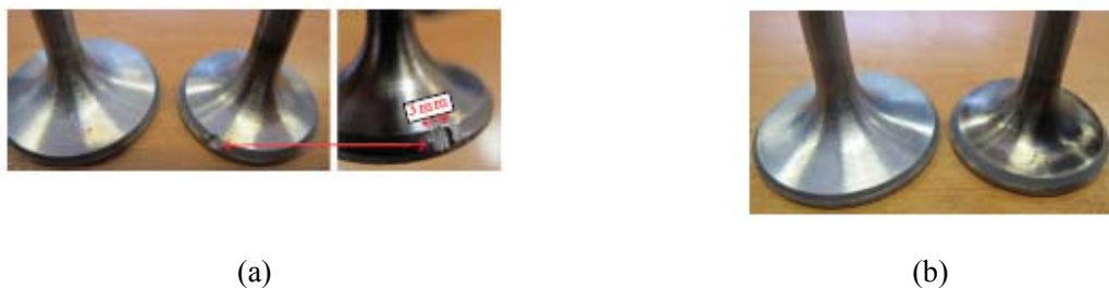
Figure 5: (a) Notched exhaust valve of cylinder No. 3 and (b) Healthy valves of cylinder No. 4. Clearance fault was simulated by lift on valves (Alhouli et al. , 2015).
