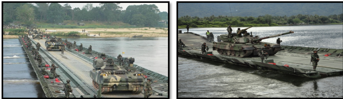
Figure 7: PFM in Tactical Heavy Raft and Pontoon Bridge configuration (Army HQ, 2016)
