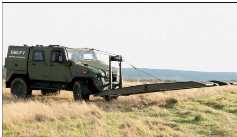
Figure 9: MTB during launching from light tactical vehicle (GDELS, 2011).
