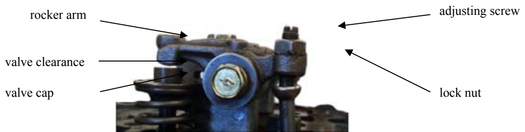
Figure 3: Valve clearance (Flett and Bone, 2016).
