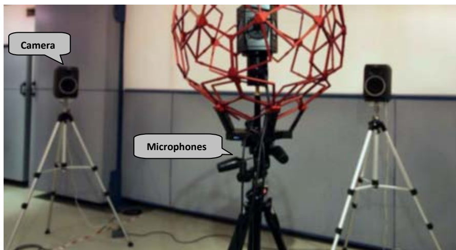
Figure 4: Array of microphone and Omni360 cameras (Source: Busset et al. , 2015).
