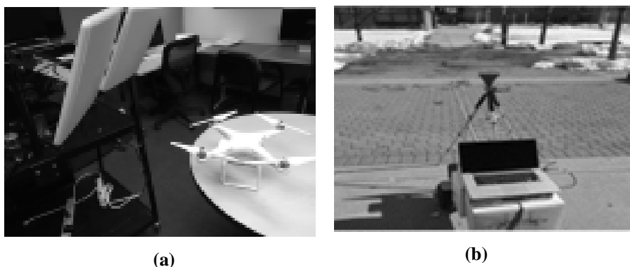
Figure 6: Experimental setup to validate the feasibility of drone detection by using an RF signal in the (a) active and (b) passive approaches (Source: Nguyen et al. , 2016).
