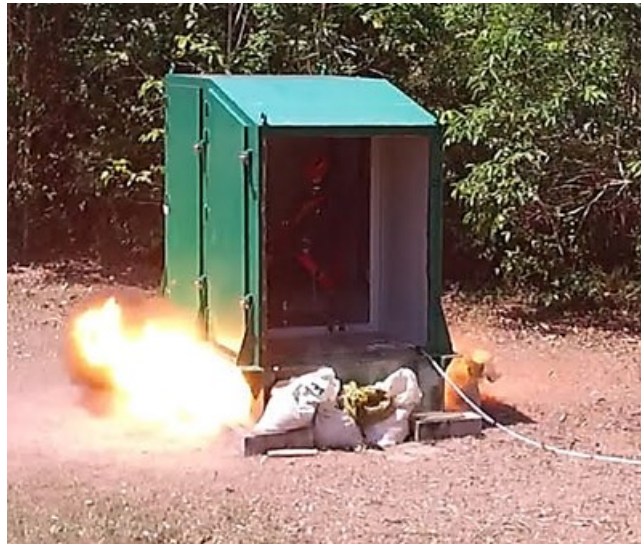
Figure 5: Blast testing of the capsule and ATD.
