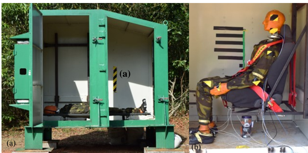
Figure 4: Dummy positioning: (a) Sitting (b) Horizontal recumbent
