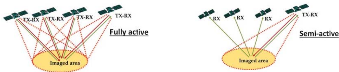
Figure-3 : Bi-static or multi-static SAR configurations (Lombardo & Pastina, 2016).
