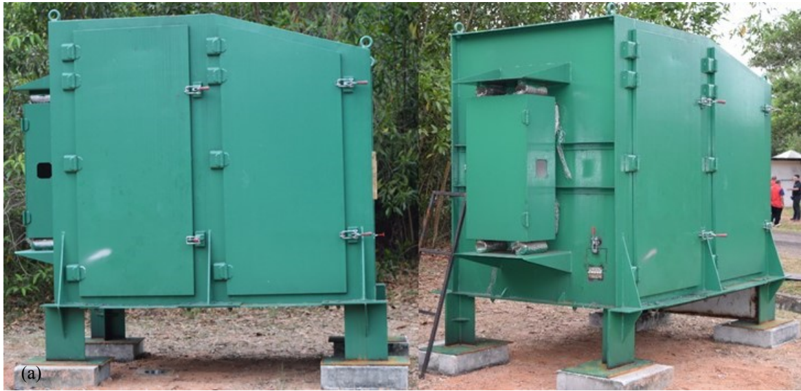
Figure 3: Fabricated blast capsule: (a) Side view (b) Rear view.
