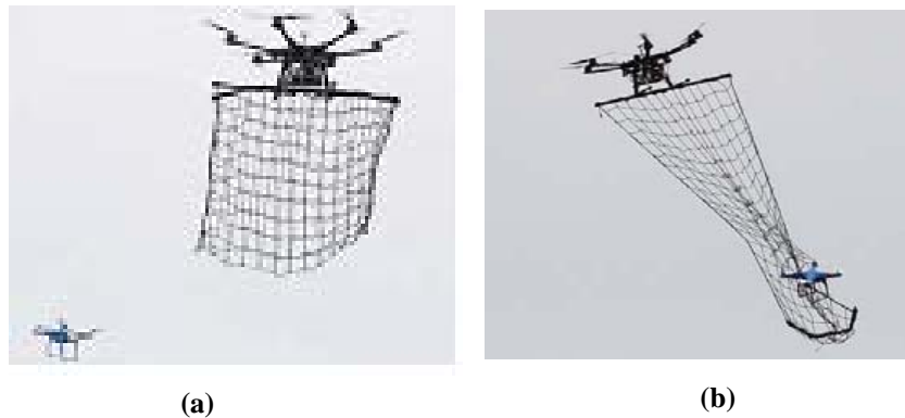
Figure 8: A Malou Tech MP200 interceptor UAV: (a) A net to intercept the drone. (b) Interceptor catching the intruding drone (Source: Humphreys, 2015).
