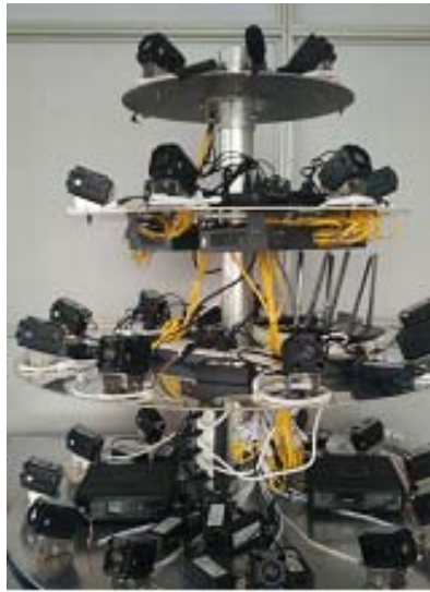
Figure 7: System view of a camera array coupled with microphones mounted on the frame for large-scale surveillance (Source: Liu et al. , 2017).
