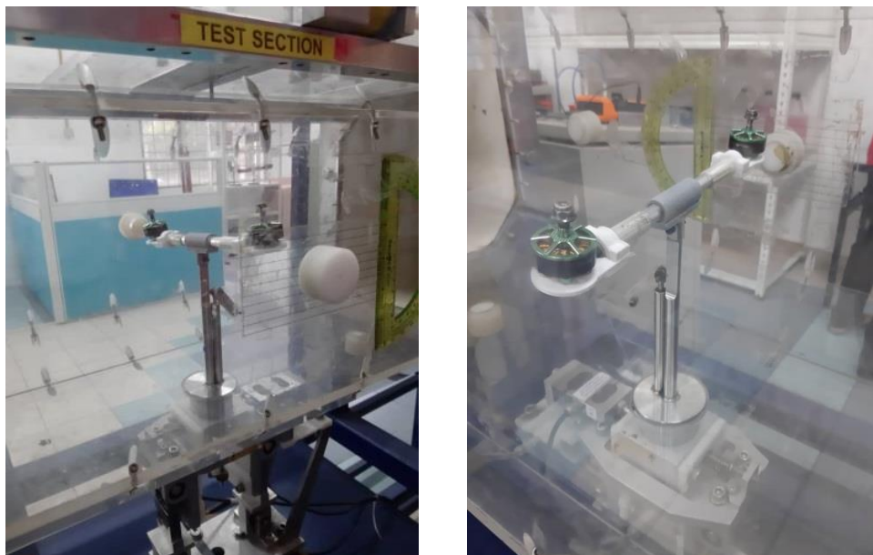
Figure 6: Subsonic wind tunnel test section and test setup arrangement for motor fairings.
