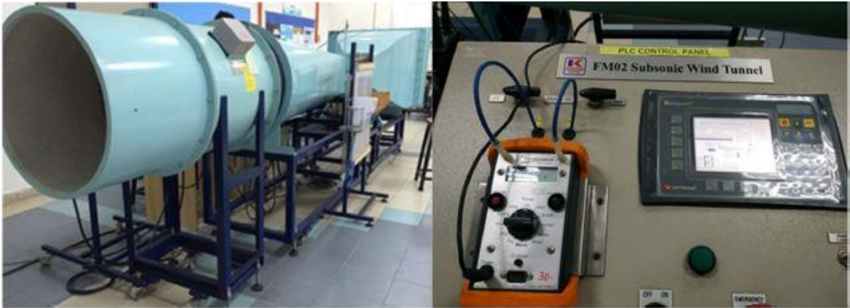
Figure 5: Subsonic wind tunnel and its control panel.
