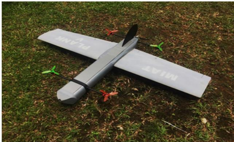
Figure 2: SLT VTOL UAV fabricated in-house.
