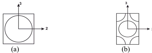
Figure 1: Example of RVE to represent homogenous of material unit cell on: (a) Square packed array (b) Hexagonal packed array (Aboudi et al. , 2013).
