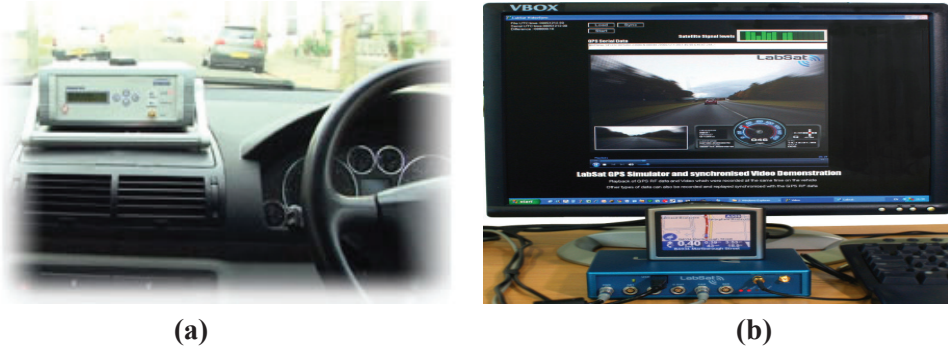
Figure 4: Commercially available GNSS record and playback systems: (a) Spirent's GSS6400. (b) LabSat 2.
