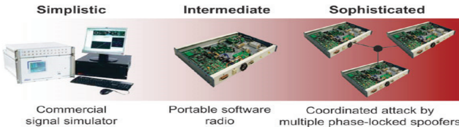
Figure 3: The spoofing threat continuum; simplistic, intermediate and sophisticated spoofing attacks. (Source: Hanlon et al. (2009)).
