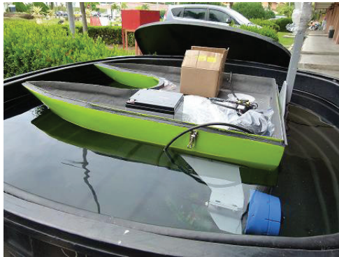
Figure 8: Buoyancy test conducted to determine the prototypes' displacements at various drafts.
