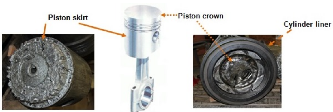
Figure 2: The separated piston crown and skirt.
