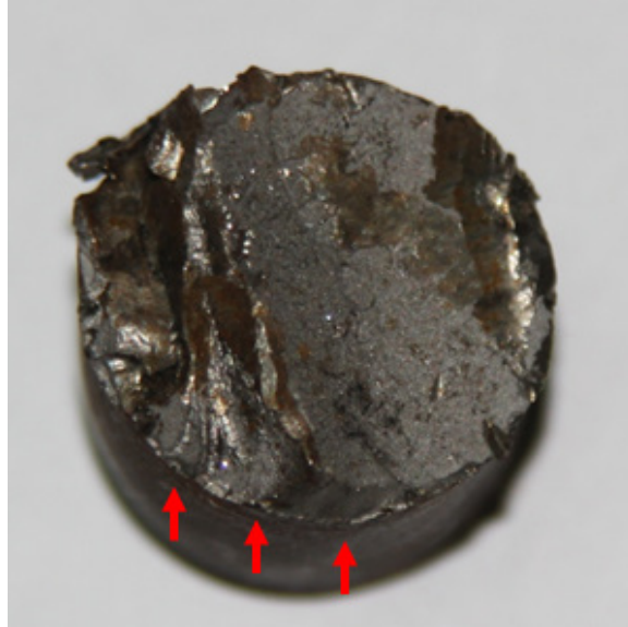
Figure 5: The fracture surface of valve stem no. 1.
