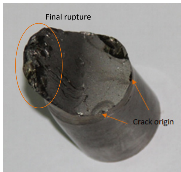
Figure 9: The fracture surface of valve stem no. 3.
