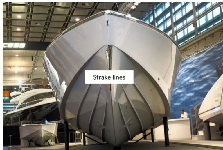
Figure 1: Strake lines running along the underwater hull of a boat. (Source: Boats, 2024)
