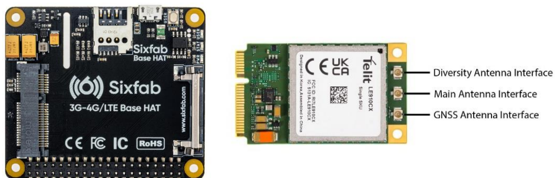
Figure 1: Sixfab 3G-4G / LTE Base HAT and Telit LE910C4-AP LTE modem.
