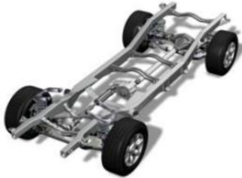
Figure 1: Ladder frame chassis. (Source: Ren et al. , 2005)
