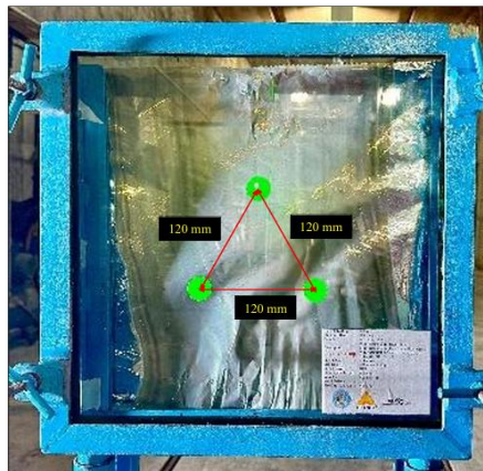
Figure 3: A sample measuring 500 mm × 500 mm with fixed striking points at distance of 120 mm.
