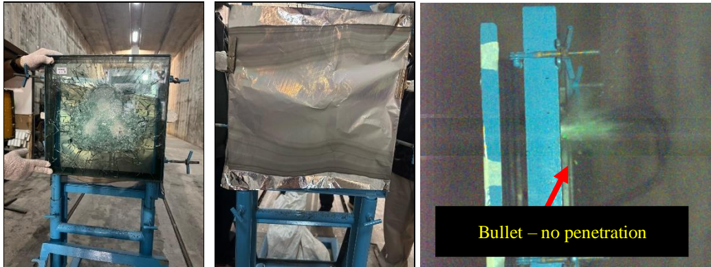
Figure 7: Double laminated glass clad with 6 mm polycarbonate at the back.
