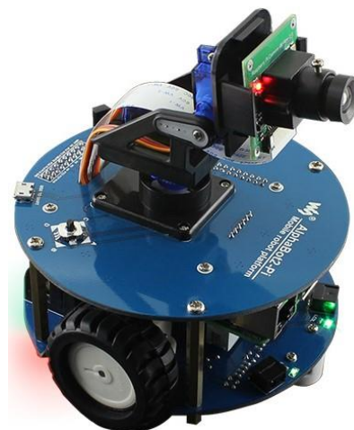
Figure 1: The AlphaBot2-Pi mobile robot platform showing its two layer construction and differential drive configuration.
