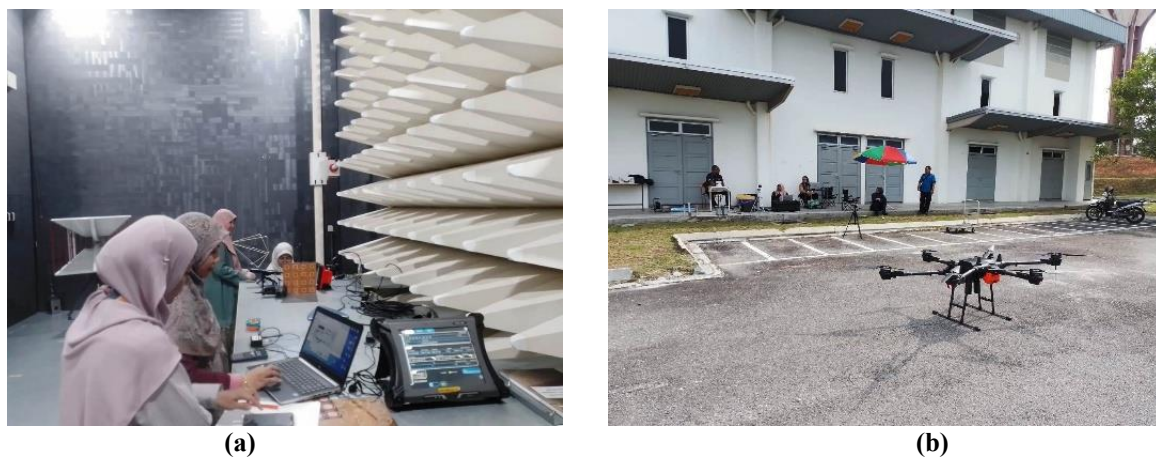
Figure 14: GNSS jamming and spoofing tests conducted by the Geospatial Technology Unit, STRIDE, through (a) GNSS simulation and (b) field evaluation.
