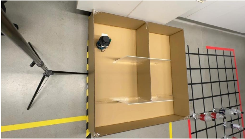
Figure 5: Custom built cardboard maze used as the experimental environment for SLAM evaluation.
