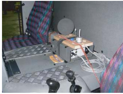
Figure 1: Heat Stress Equipment consist of Black globe bulb thermometer, natural wet bulb thermometer and dry bulb thermometer.
