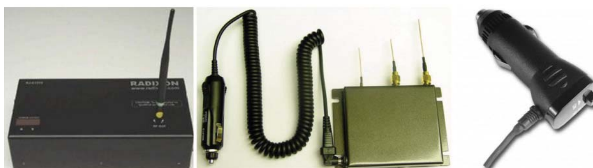
Figure 3: GNSS jammers found during casual browsing of the internet. The sources of the figures are not given for obvious reasons. Readers are reminded that GNSS jamming is illegal.
