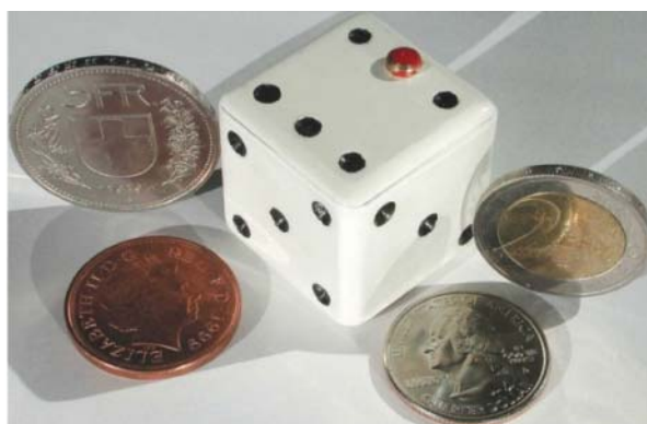
Figure 2: A GNSS jammer hidden on a dice. (Source: Last (2008))
