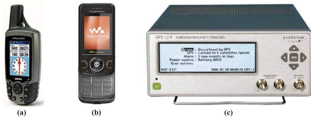
Figure 1: GPS receivers evaluated in this study: (a) Handheld: Garmin GPSmap 60CSx (b) Handphone: Sony Ericsson W760i (c) Fixed: Pendulum Instruments GPS-12R.
