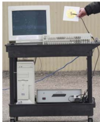
Figure 5: A homemade GNSS simulator. (Source: Johnston & Warner (2004))
