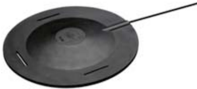
Figure 2: Triaxial seat accelerometer 4515-B. Figure 3: Bruel & Kjaer 4447 WBV meter.
