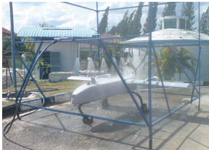
Figure 3: Rain test being conducted on the UAV
