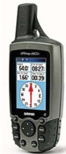
Figure 1: A Garmin GPSmap 60CSx handheld receiver.
