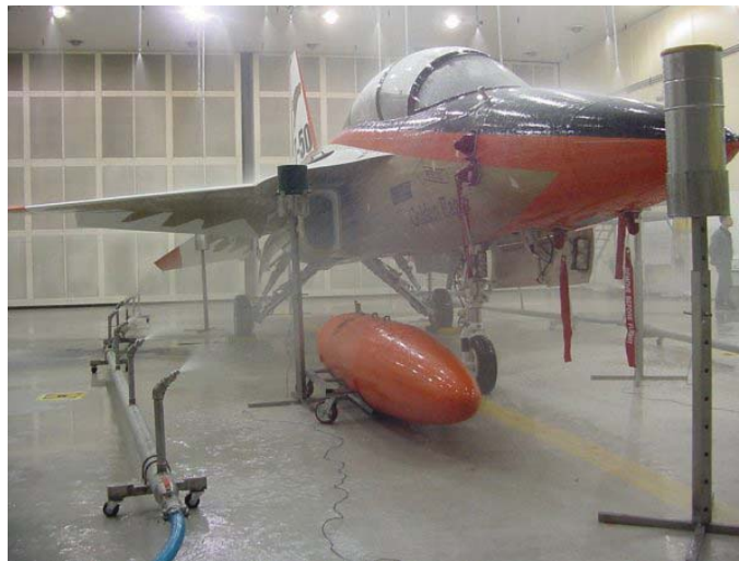
Figure 1: Rain test done on a T-50 aircraft (Source: KAI Structural Test Lab, 2010)
