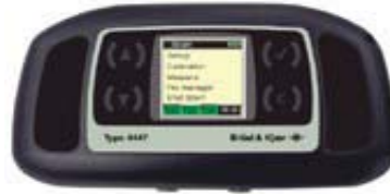
Figure 2: Triaxial seat accelerometer 4515-B. Figure 3: Bruel & Kjaer 4447 WBV meter.
