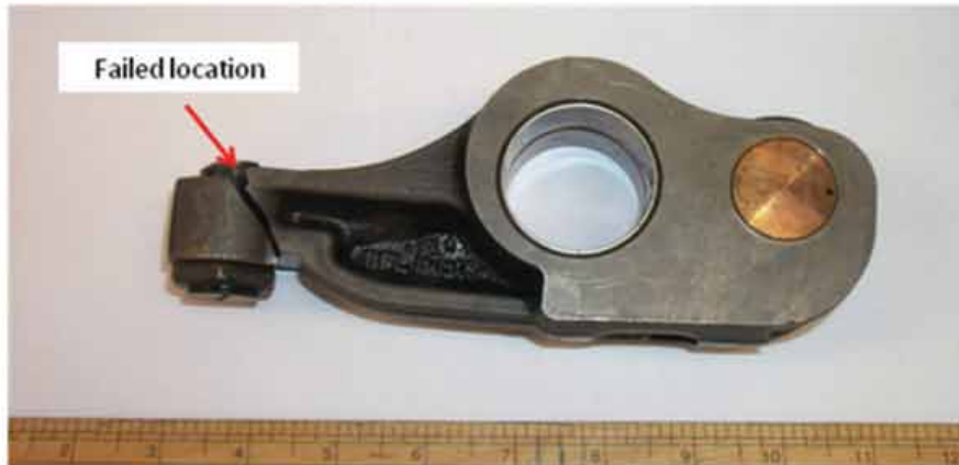
Figure 1: The failed rocker arm.
