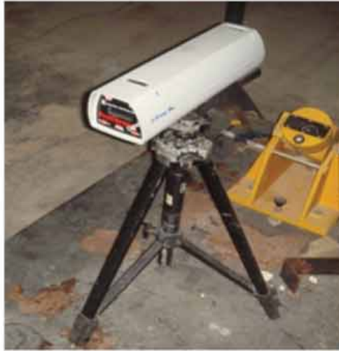
Figure 2: Portable velocity chronograph.
