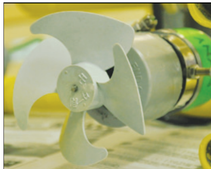
Figure 8: A completed thruster, consisting of a Mabuchi DC motor with PVC housing.
