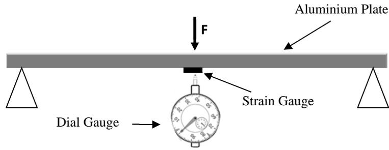
**Figure 3: Schematic of the experimental set-up for bending test.**
