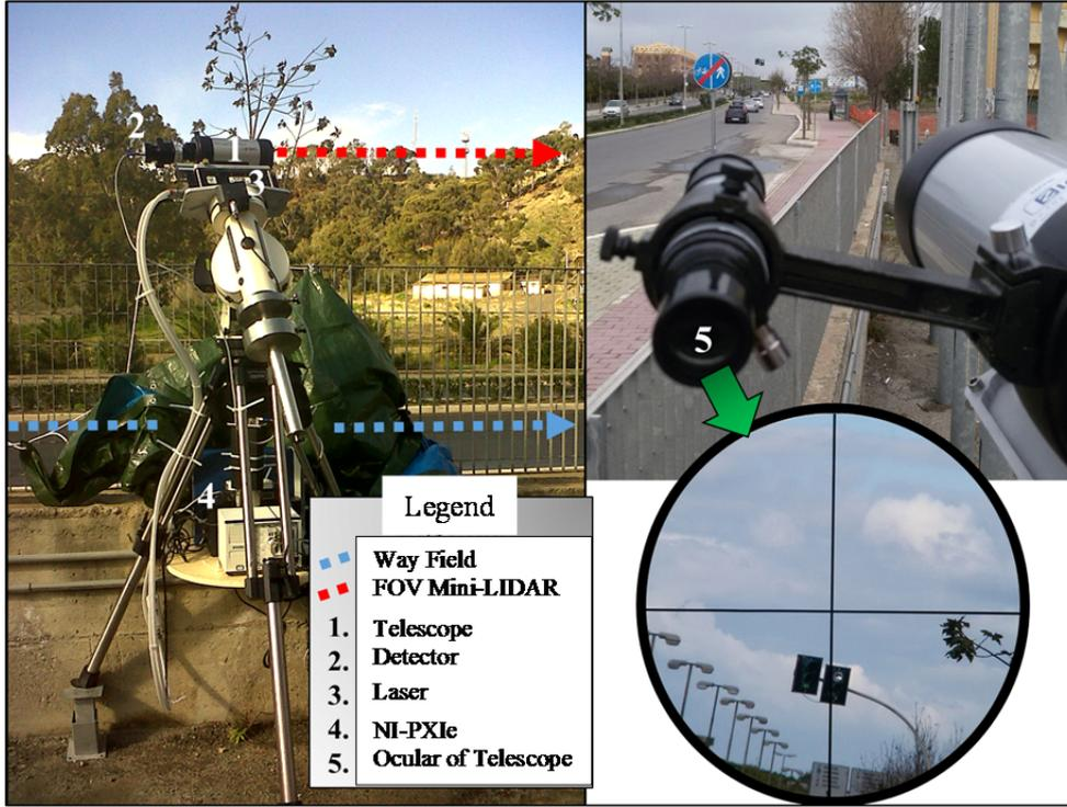
Figure 1: The developed mini-LIDAR system.
