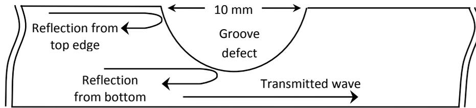
**Figure 10: Expected reflection waves around defect.**
