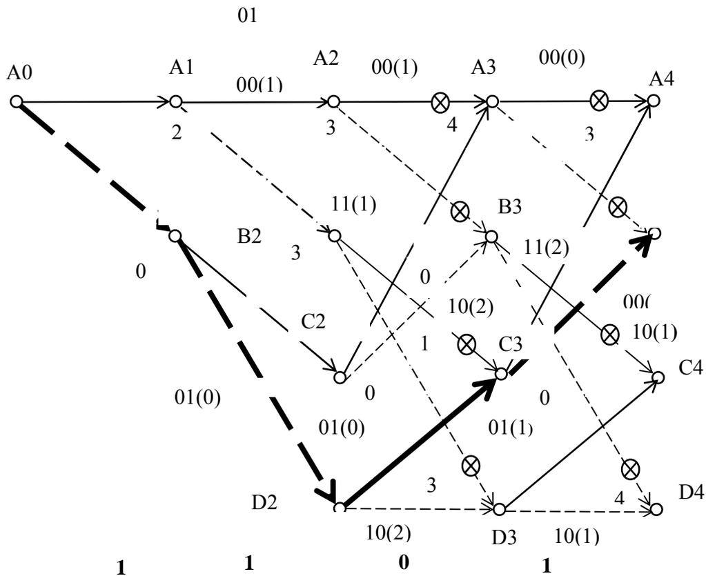
Figure 4: Working principle of Viterbi algorithm without noise (Simon *et al.*, 2012).
