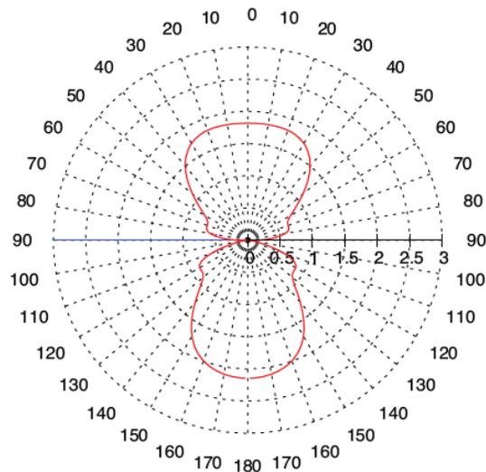
**Figure 5: Example of the radiation pattern of a quad helix antenna operating in endfire and backfire modes simultaneously (Source: Slade, 2015)**
