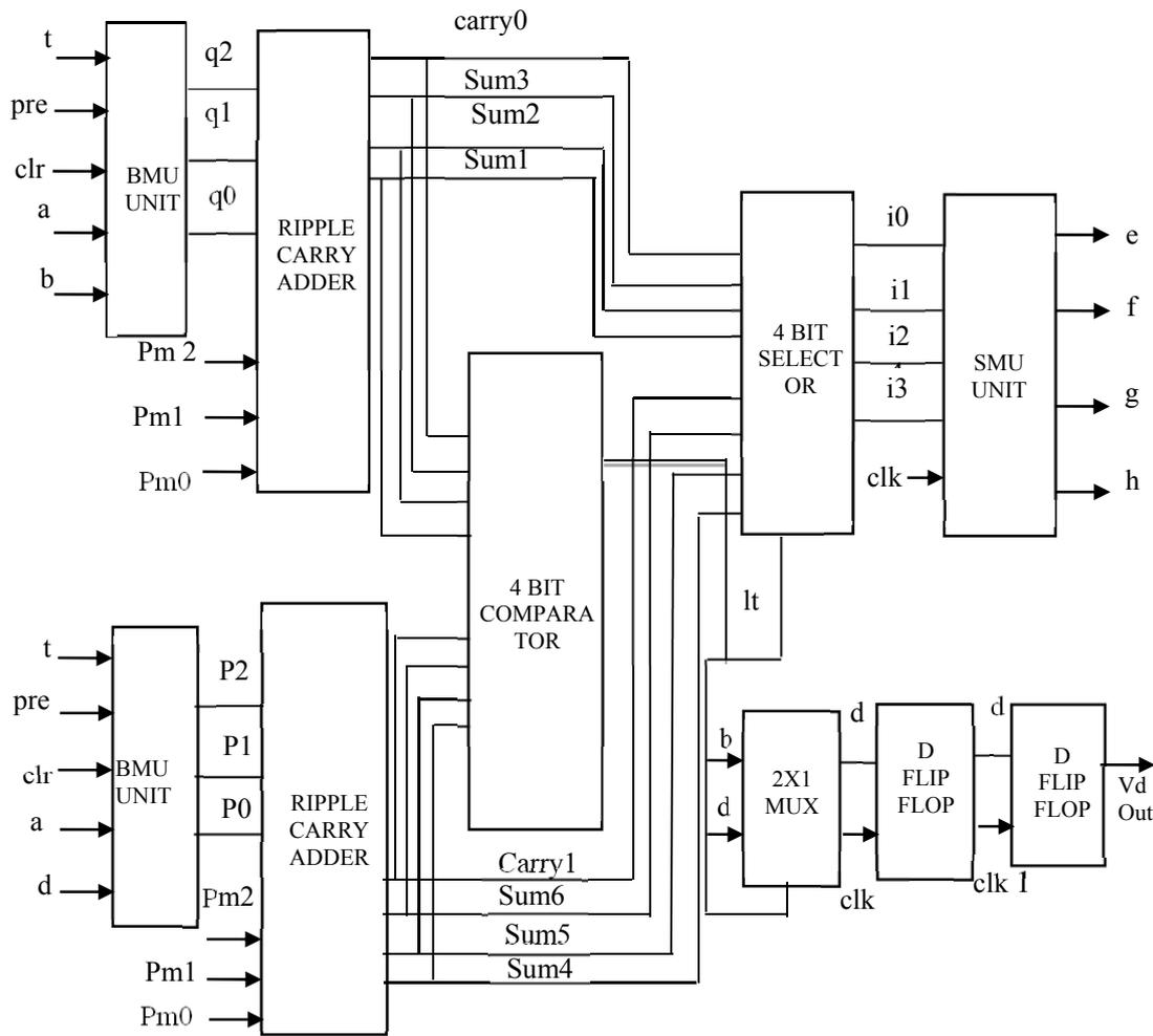
Figure 6: Block diagram of the proposed Viterbi decoder.
