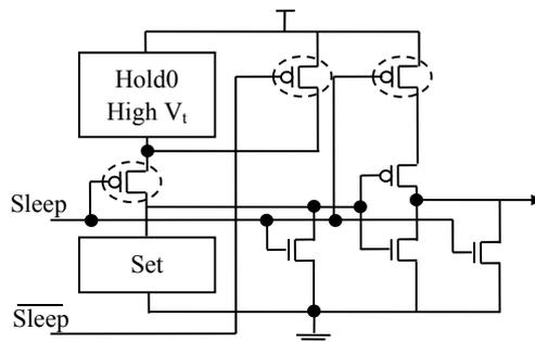
Figure 5: General structure of the MTNCL design (Sudhakar *et al.*, 2016).
