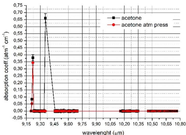
**Figure 7: Acetone absorption spectra**
