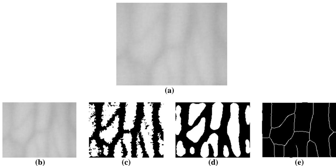
**Figure 9: Resulting vein image for each sub-module for the proposed method: (a) Original vein image. (b) Resampling. (c) Segmentation. (d) Median filtering. (e) Thinning.**
