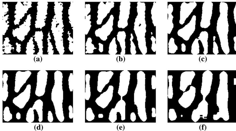
**Figure 6: Resulting vein images for different median filter size: (a) 3x3; (b) 7x7; (c) 11x11; (d) 15x15; (e) 19x19; (f) 23x23.**
