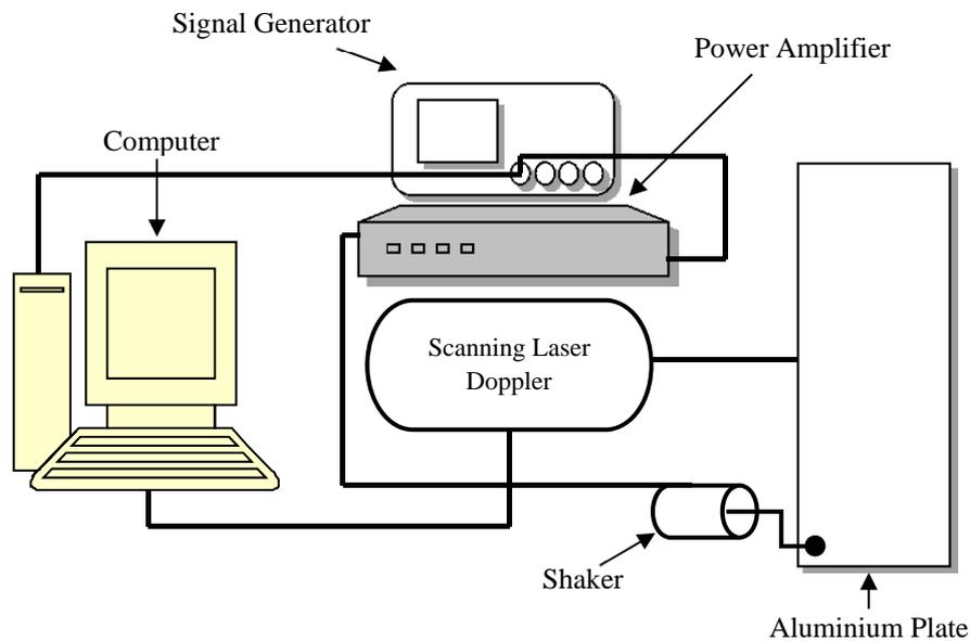
**Figure 1: Test setup for modal analysis.**
