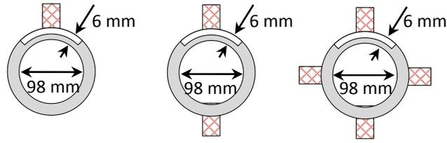
(a) 1 transducer (b) 2 transducers (c) 4 transducers
