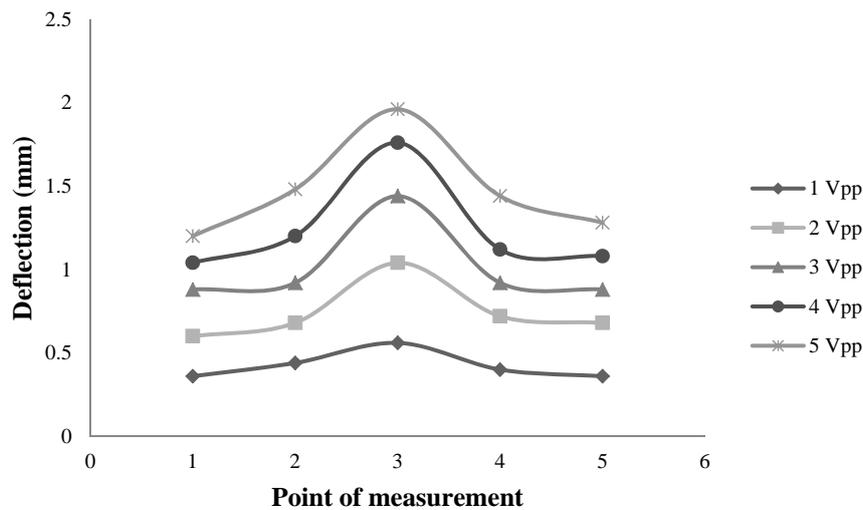
**Figure 9: Deflection results at 5 measurement points due to 1<sup>st</sup> vibration mode frequency excitation excited by various excitation power levels.**
