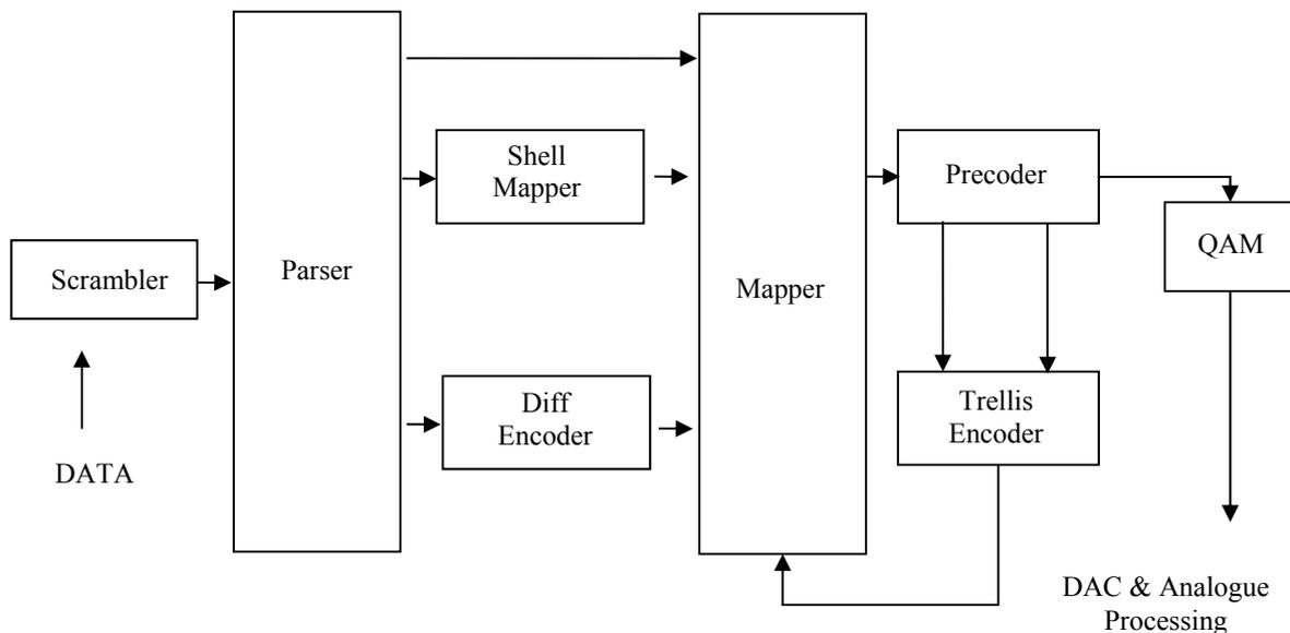
**Figure 1: Functional diagram of a V.34 transmitter modem.**
