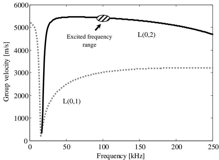
**Figure 5: Group velocity dispersion curves of in aluminum pipe at 6 mm thickness.**
