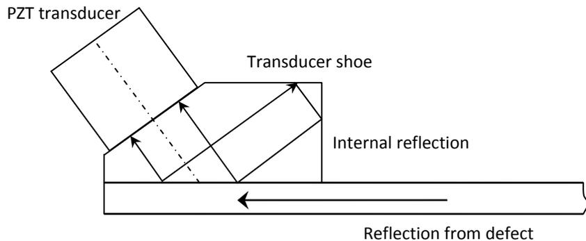
**Figure 11: Expected internal reflection waves in transducer shoe.**
