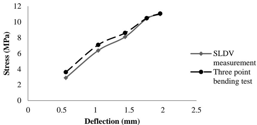
**Figure 10: Comparison of the stress measured by single head SLDV and calculated based on three point bending test.**
