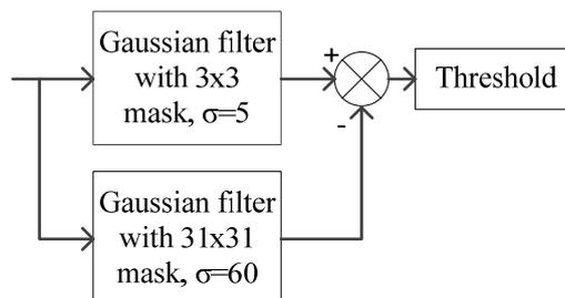
Figure 5: Block diagram for image segmentation.
