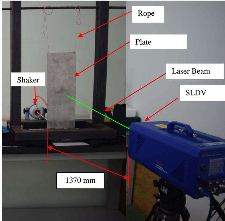
**Figure 2: Single head SLDV experimental set-up.**
