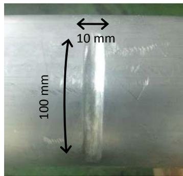
**Figure 2: Circumferential defect at 3 mm depth in pipe.**
