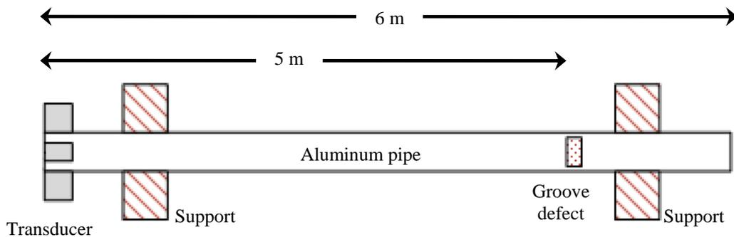
**Figure 3: Defect location.**
