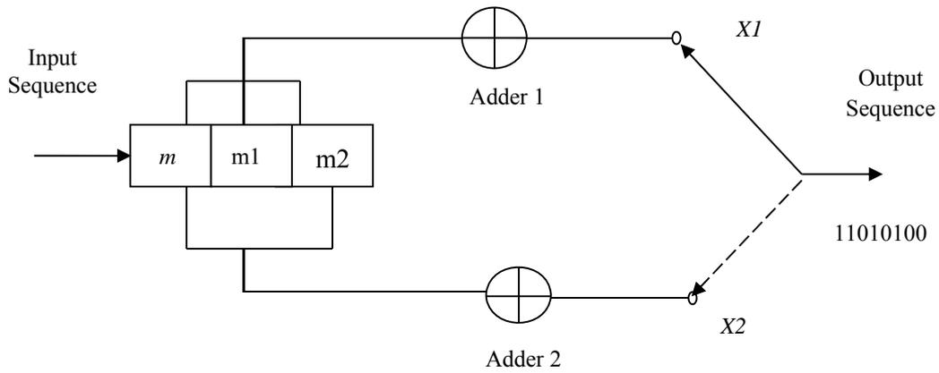
Figure 3: Functional behavior of encoder.
