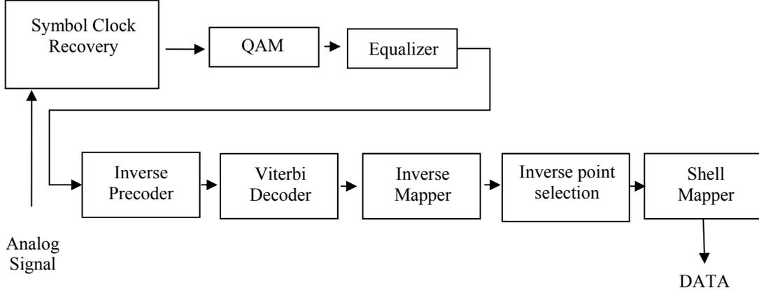
**Figure 2: Functional block diagram of a V.34 receiver.**
