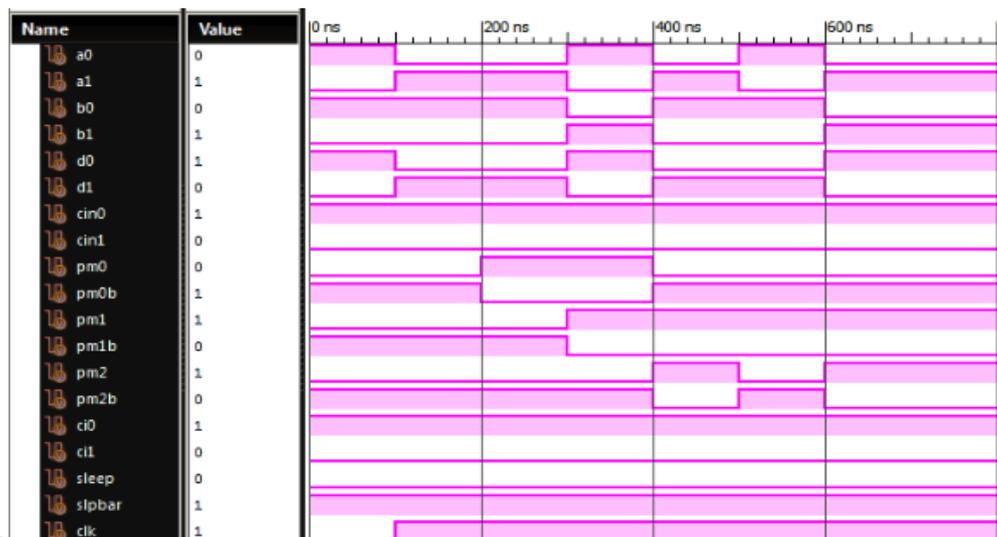
Figure 8: Output waveform of Viterbi Decoder.
