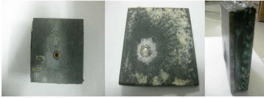
Figure 7: Impacted mild steel tested (front and back face).
