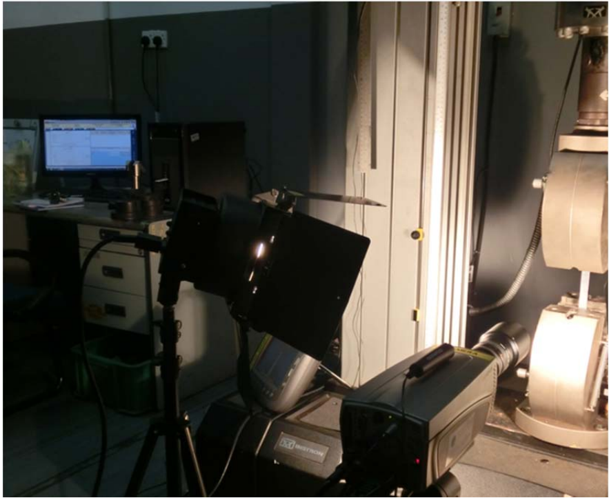
Figure 3: Digital Image Correlation measuring in plane strain.
