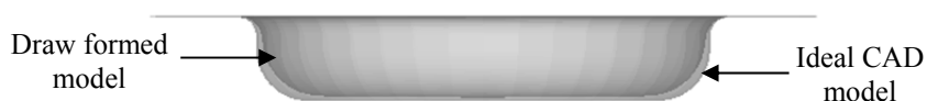
Figure 4: Comparison of geometrical shape between ideal CAD and FE draw formed developed model.
