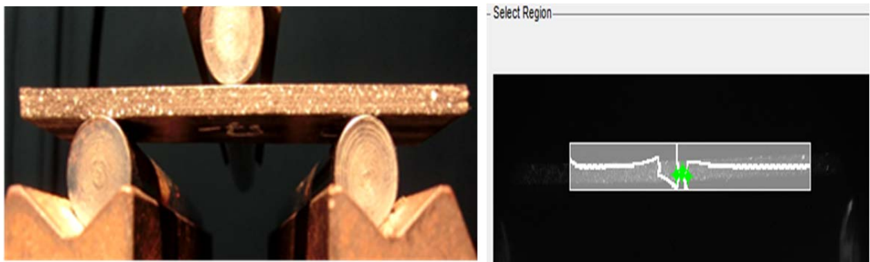
Figure 13: Three point bending at 0N load Hybrid Composite CFRP/GFRP and region of interest for bending deflection computation.
