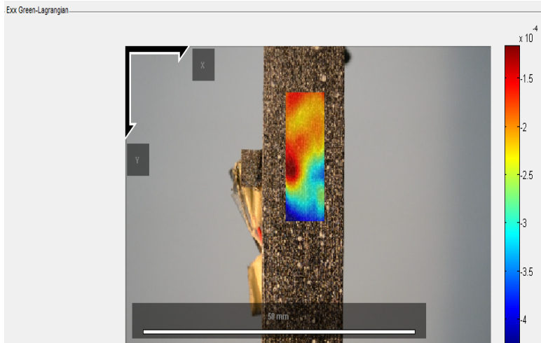
Figure 16: Contour of strain xx (transverse), \epsilon_{xx} CFRP 0° at 5,000 N.
