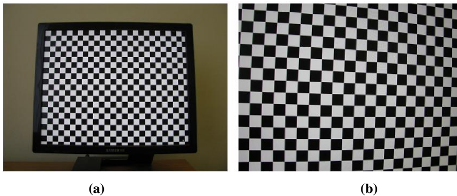
Figure 5: Image of an (a) incorrect and (b) correct calibration target.
