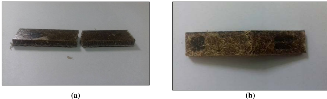
Figure 7: Izod impact samples after the test; (a) complete break; (b) partial break.
