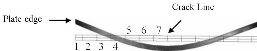
Figure 8: Example of the first mode shape of the aluminium plate.
