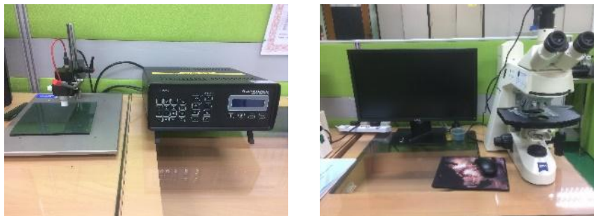
Figure 5: Four-point probe and image analyser that been used in characterisation process.
