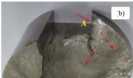
Figure 5: (a) The fracture surface was cut into three pieces. The red arrow indicates the starting point and the directions of the propagation. (b) Point A. (c) Point B.
