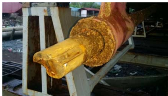
Figure 1: Propeller shaft failure.
