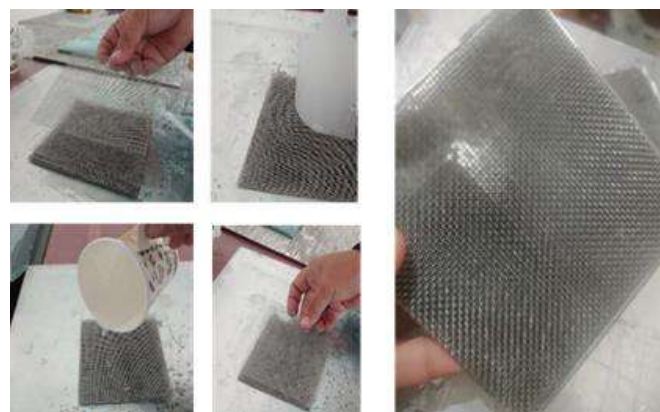
Figure 2: Laminating process of wire mesh composite.
