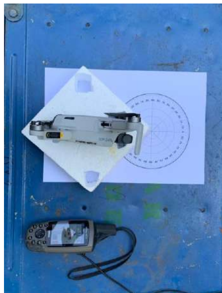
Figure 3: The rotational angle measurement with 0, 45 and 90° for the upright position.
