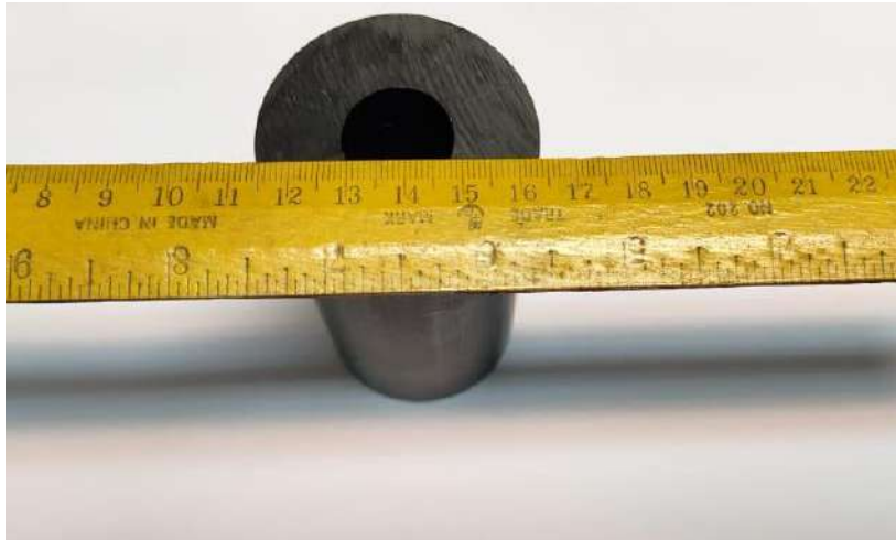
Figure 1: Double-base solid propellant with hollow cylinder shape.
